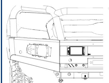
Position bull bar with vertical adjustment so radar is central to bullbar opening and tighten bullbar. Horizontally align the radar behind the front face of the bar at rectangular hole, ensuring the radar is paral-
